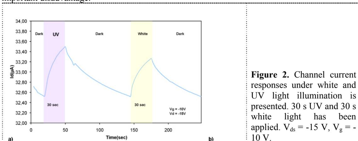
**Figure 2.** Channel current responses under white and UV light illumination is presented. 30 s UV and 30 s white light has been applied.  $V_{ds} = -15 \text{ V}$ ,  $V_g = -10 \text{ V}$ .
