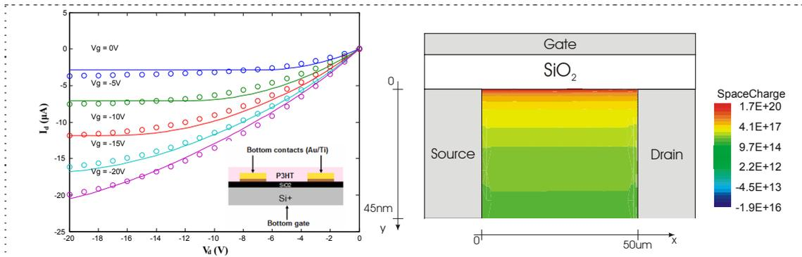
**Figure 1.** Left: Measured (circles) and simulated (lines) output characteristics of an OFET with P3HT spun out of toluene with a channel length of 20  $\mu\text{m}$  and  $W/L = 13,350$  on 80 nm silicodioxide. Inset: schematic picture of the transistor structure (cross-section) adopted in our studies. Right: Space charge distribution at  $V_g = -10\text{V}$ ,  $V_d = -15\text{V}$
