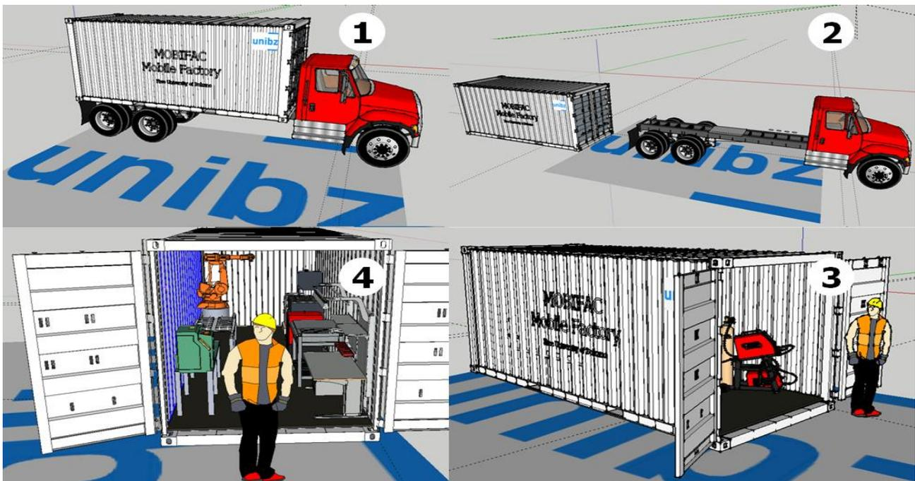
Fig. 1 Draft of the Mobile Factory concept (1. delivery via ship or truck, 2. unload on-site, 3. setting up on-site, 4. setting up of process modules)
