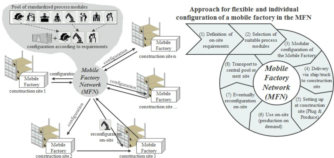
Fig. 2 Structure and configuration approach in the MFN
