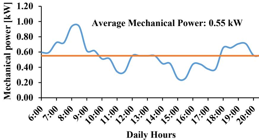
Fig. 5. Daily mechanical power produced by each PaT
