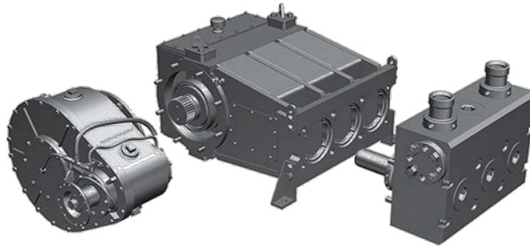
Figure 1: typical layout of a motor pump: mechanical power transmission (left), power end (centre) and fluid end (right) <http://www.jasonoandg.com/product/600s-triplex-plunger-pump.htm>
