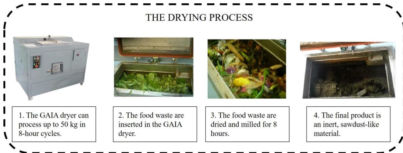
Figure 1. The process of drying and milling of food waste in a commercial GAIA dryer.
