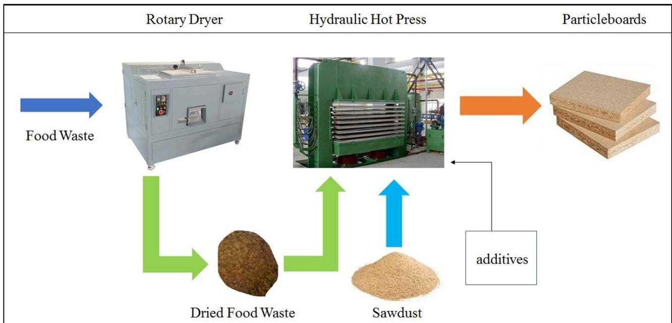
Fig. 4. Proposed concept for particleboard production from mixtures of wood sawdust and dried food waste (Source: Vakalis et al., 2017)
