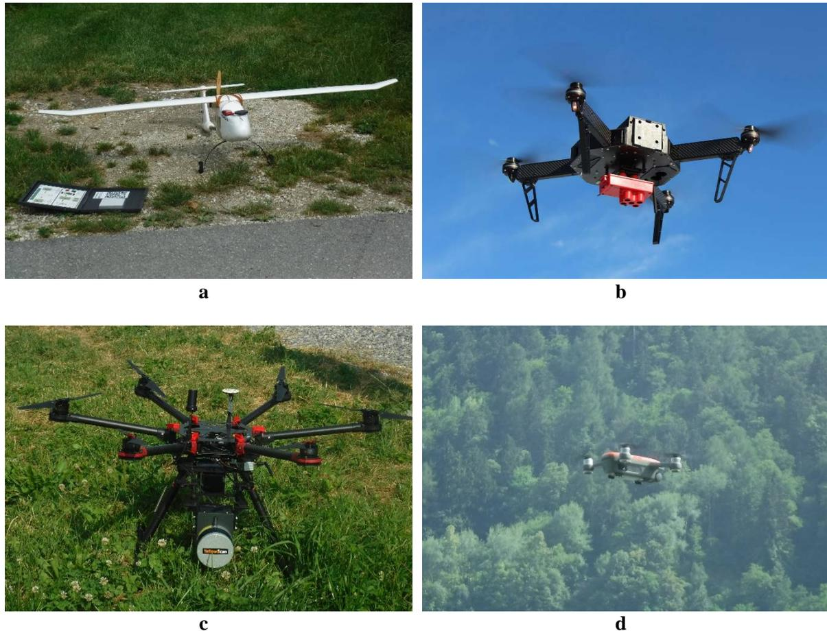
**Figure 1.** The UAVs developed during the WEQUAL project. Each one is used for different tasks and it is equipped with specific sensors: a) MAVTech AGRI-1900 for multicamera or RGB survey for large surfaces; b) MAVTech Q4E for multicamera or RGB survey for small surfaces; c) DJI S900 for LiDAR surveys; d) DJI SPARK for video recording.
